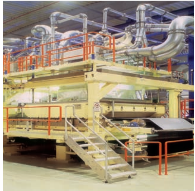
Airlaid production plant of the company Concert GmbH – manufacturer of airlaid cellulose nonwoven fabrics
