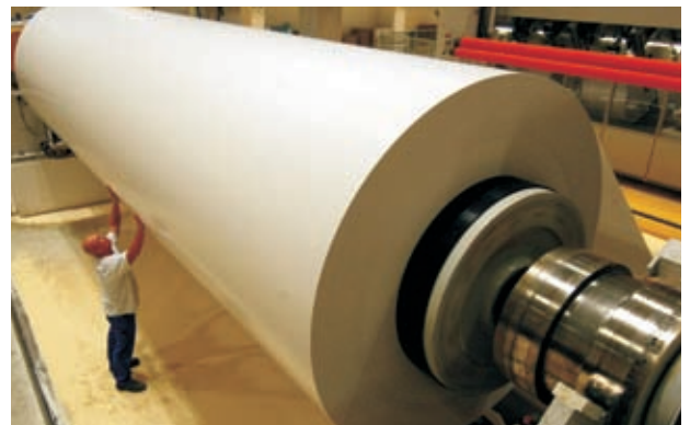
Tambour at the end of the paper making machine 4 at the company LEIPA Georg Leinfelder GmbH
